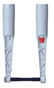
**Rebound** controls the rate of speed at which the fork extends after compressing.
