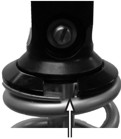
INCORRECT SPRING ORIENTATION
