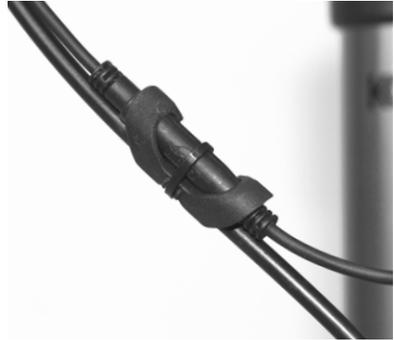
5. Install a cable clip near the head tube on the front sensor cable and the other cable.
