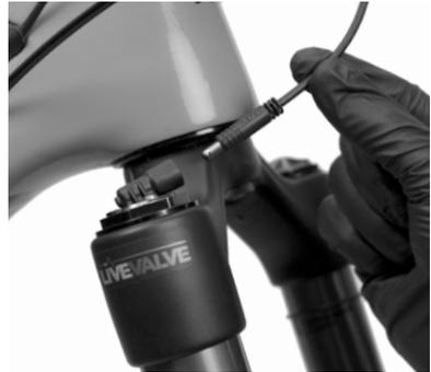
9. Compress the fork to bottom out and make sure there is a strain relief loop in the cable and that it can move freely as the fork goes through the travel. Check to make sure the cable is oriented to clear the fork brace without pinching.
