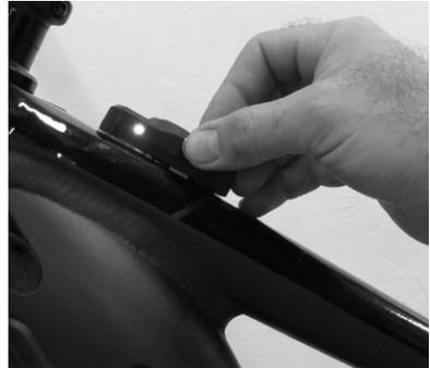
6. When the calibration is complete, the LED will change color and display a series of blue flashes.
