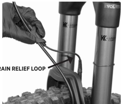
4. Install a zip tie around the center of the sensor clip.
