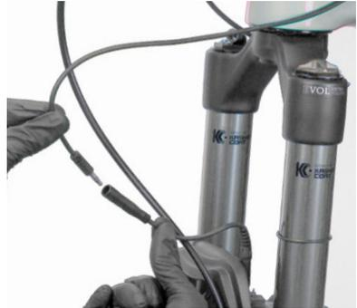
3. Make sure to orient the sensor connector on top of the brake line and closest to the fork. Snap the sensor clip to brake line first, and then snap it to the sensor connector. There **must** be a strain relief loop in the cable so it can move freely as the fork goes through its travel.
