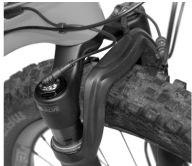
10. Install a cable clip near the head tube to attach the front solenoid cable to the other cable.
