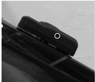
4. Position a magnet over the sensor on the controller as shown.
